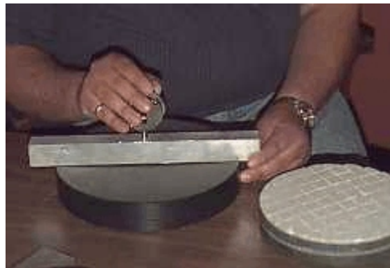
Figure 3: A simple spherometer using the economy dial indicator and an aluminum bar 1 1/4" square and 14" long. Once zeroed, this setup can read the sagitta directly.
