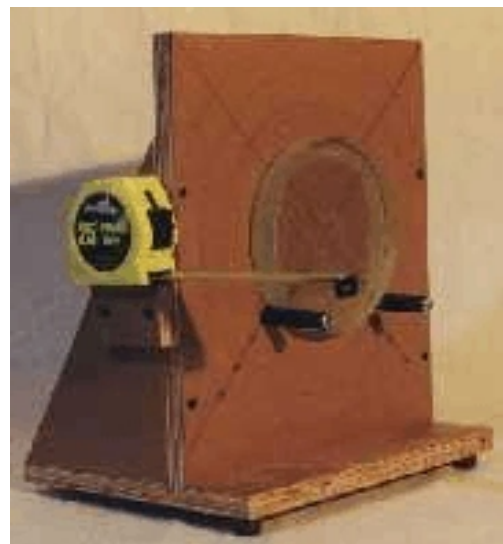
Figure 2: The companion, adjustable Mirror Test Stand with a 6" Mirror. The attached steel rule makes Radius and Curvature easy for a single person.
