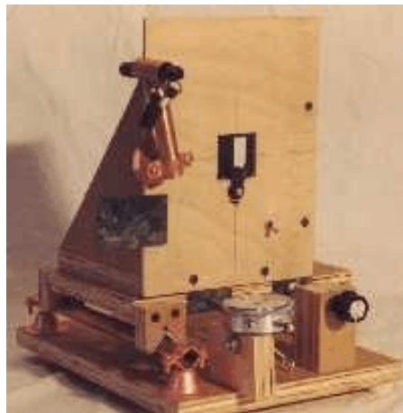
Figure 1: The Foucault Tester described in this article, made from easily obtainable parts with only common hand tools.
